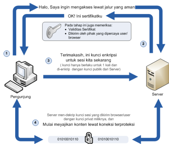
Gambar Error! No text of specified style in document..3 Simulasi cara kerja HTTPS
